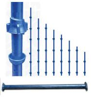
A.Verticals / Standards: Pipe 40 NB (OD 48.3 mm ) ERW mild steel medium / heavy class The connection points are set at every 500 mm vertical interval of standard vertical member. Top cups are made out of malleable cast Iron. Bottom cups are made out of MS forging. Spigots are available for continues connections. Verticals are available in standard sizes.
