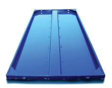
Purpose: To cast floor, beams etc. Components & Features: Manufactured from 14G (2 mm) hot rolled MS sheet. Pressed on four sides and provided with box stiffeners. Provided gusset plates on corners for rigidity.
